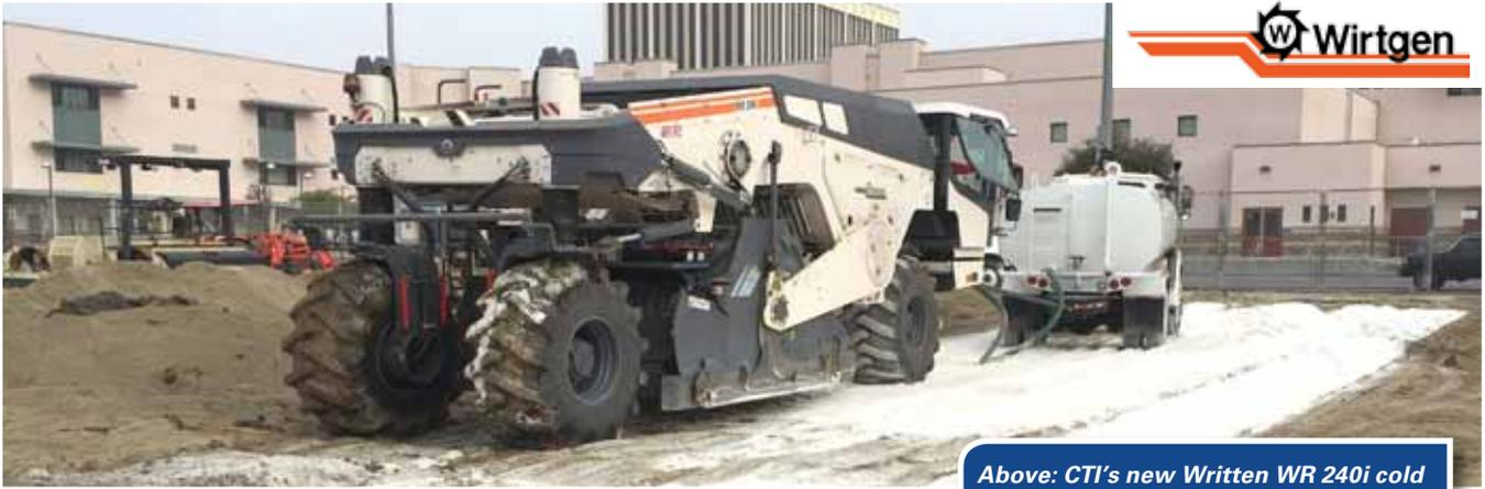
Above: CTI's new Wirtgen WR 240i cold recycler/soil stabilizer working on an LAUSD project.
